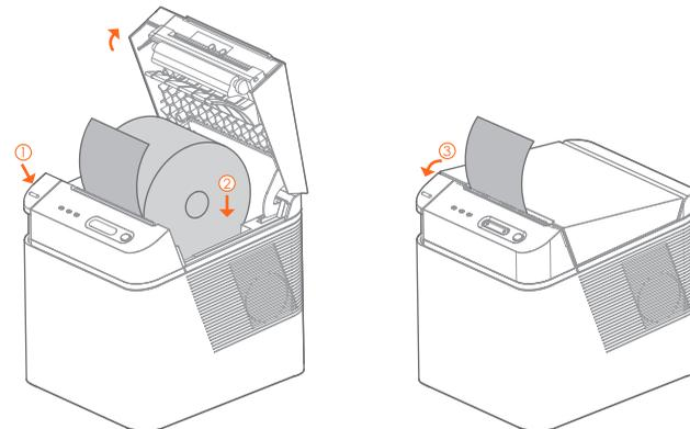
**1** Press the door cover button to open the printer flip cover.
